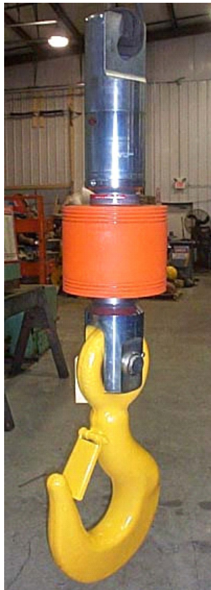
Insulated, 60T, NASA shuttle maintenance operations
